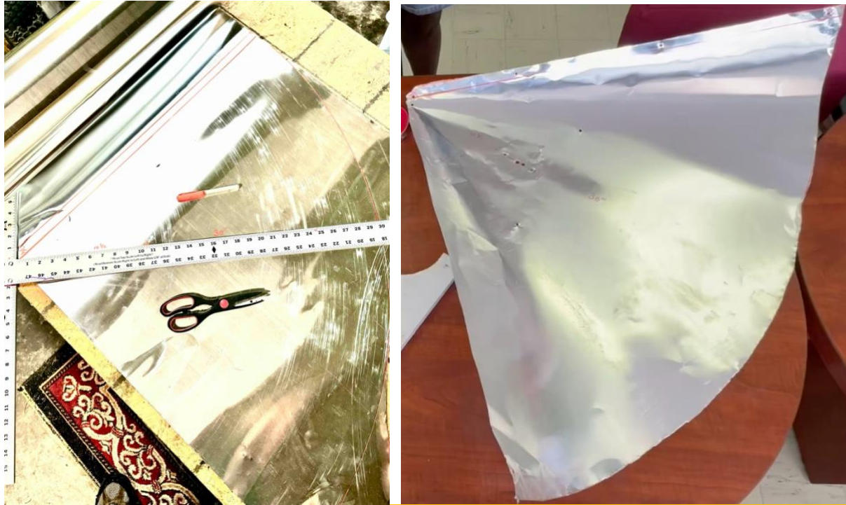
Fig 4: Draw \frac{1}{4} of a circle on your flashing with a ruler (left). Screw reference point through the flashing and board holding the flashing. Draw an arc of circle the width of the flashing. Use a permanent marker. The flashing should be 20-inches or wider. Arc should go one inch further than a quarter-circle, so there will be an overlap when bolting the cone together. Use scissors to cut the flashing, creating a big semi-circle (right).
