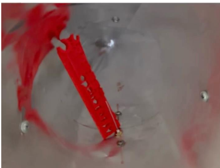
Fig 12: The assembled cone-horn opening, showing the feed probe in front of a short red ruler (left). The feed probe is 10.5-inches from the point of the cone. At right, we zoom in on the feed probe, which is the thin silver wire. The heads of the wood screws for attaching the cone to the mount are visible on the sides.
