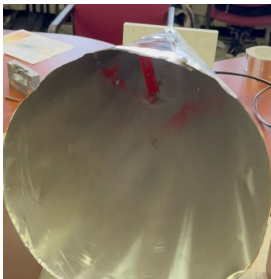
Fig 12: The assembled cone-horn opening, showing the feed probe in front of a short red ruler (left). The feed probe is 10.5-inches from the point of the cone. At right, we zoom in on the feed probe, which is the thin silver wire. The heads of the wood screws for attaching the cone to the mount are visible on the sides.
