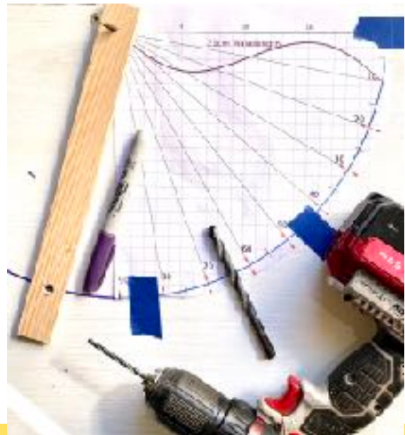
Figure 5: Make the protractors on one sides..The protractor template is taped in place and use an 1/8 inch drill bit to put two holes, separated by about a half inch.
