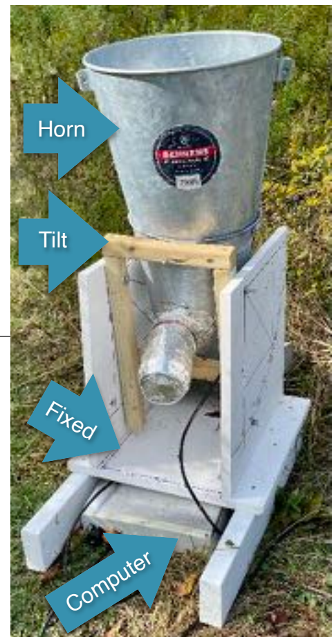
Figure 1: Completed horn radio telescope. The total height of the telescope is about 3 feet (1m). The fixed part is white and the tilting part is brown.
