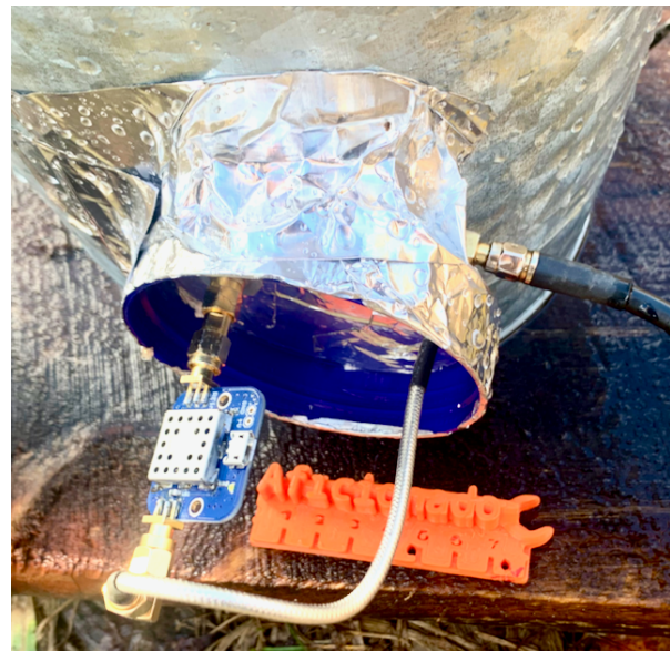
Figure 10: Inside view of the peanut butter jar lid with amplifier and connecting SMA cables. This example shows the GPIO Labs amplifier, which fits in the same place as the NooElec amplifier.
